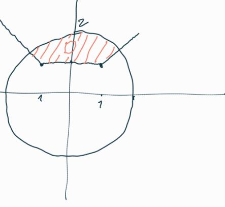
$$\bar{y} = \frac{1}{m(D)} \left( \iint_D \rho(x, y) y \, dx \, dy \right)$$
